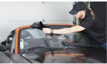
The stripe and windscreen must be completely wet. Lay the strip approximately without seeking to stick it.
