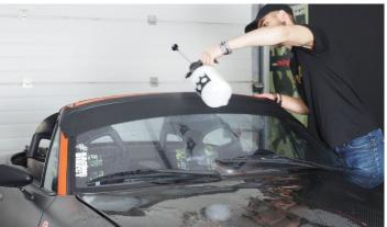
Wet the top of the sun visor to protect it from scratches that may be occasioned in the following steps.
