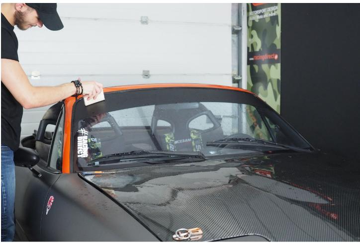
Spend 10 minutes to remove the last bubbles. Do not hesitate to heat the stripe with a heat gun or a hair dryer to eliminate the most recalcitrant bubbles.
