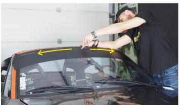
Cut along the joint with a cutter.
